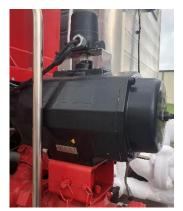
This valve actuator opens and closes the discharge valve. The discharge valve is controlled through the Discharge Valve Selector Switch on the console in the cab. The two lights indicate whether the valve is opened or closed. NOTE: The Valve is pinned opened physically.
