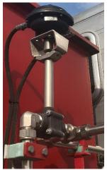
This valve opens and closes based on the unmarked lever on the console inside the cab. The intake of the valve comes from the N2 tank and the Pump and the outtake of the valve goes to the atmosphere. This valve seems to be a bleed valve for the line between the check valve for the N2 Tank and the Pump.
