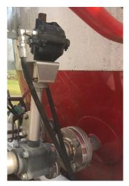
This valve opens and closes based on the Bottom Fill Valve lever on the console inside the cab. The one side of the valve goes to the N2 tank and the other side goes to the Fill Valves, Valve V4, and Valve V2. The valve when open will either have the liquid Nitrogen travel from the Fill Valves to the N2
