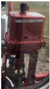
This valve actuator opens and closes a valve with the intake coming from the Pump and the outtake going to one of the intakes of a cross fittings. The button will control the valve if the Valve Control Selector Switch is set to Manual mode. If the Valve Control Selector Switch is set to Auto mode, the PLC will control the valve. If the Manual Override button is pressed, the plus and minus adjust buttons for the Temper Valve #1 on the Nitrogen Systems screen.
