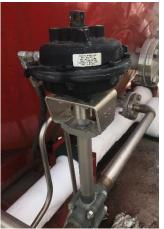
This valve opens and closes based on the Pressure Build Valve lever on the console inside the cab. The one side of the valve goes to the N2 tank and the other side goes to the Heat Exchanger on the side of the N2 Tank.
