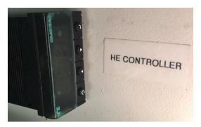
Turbine. This valve is controlled by the Omega PID controller on the door side of the console in the cab.
